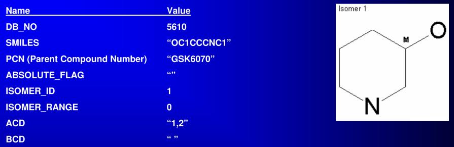
A mixture of enantiomers is present, the major of which falls within the range A%-B%. Since the identity of the predominant isomer is unknown normal bonds are used in the display with a compulsory text field descriptor ISOMER n.
